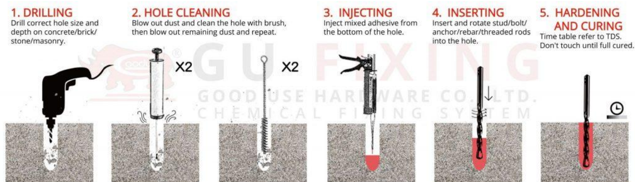
Fig. 4.8 Chemical Anchoring in Structures
