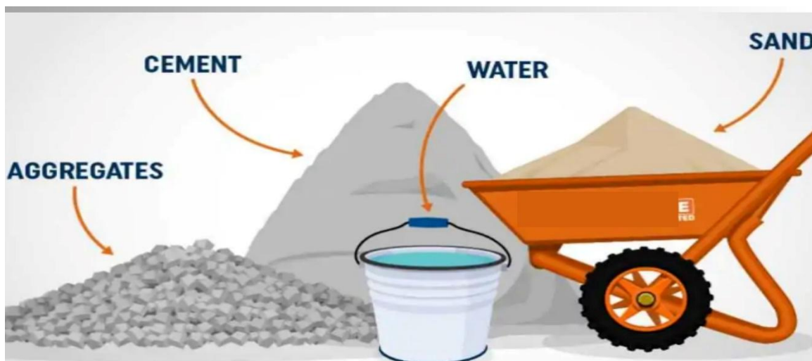
Fig. 4.2 Composition of Concrete
