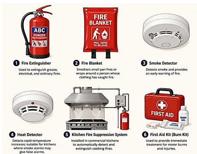
Fig. 1.12: Fire equipment in kitchen
