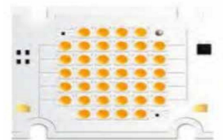
Fig. 6.3: Flexible based light engine module
