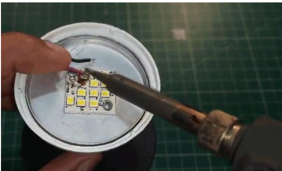
Fig. 6.14: soldering of components
