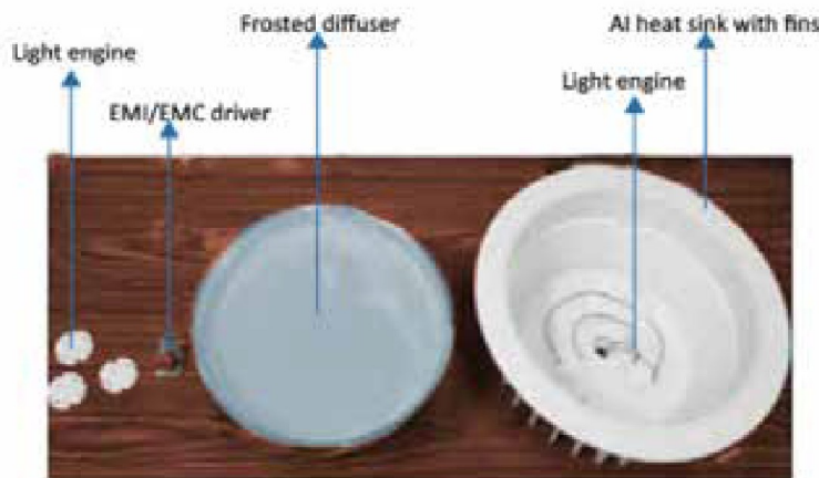
Fig. 6.24: Downlight Assembly parts
