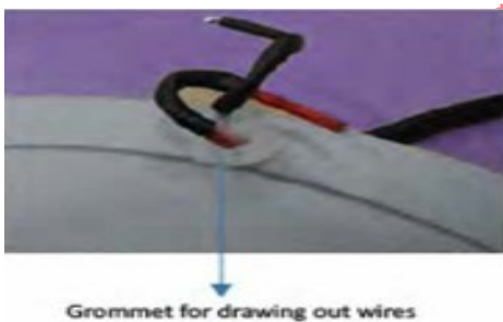
Fig. 6.29: grommet in round panel light
