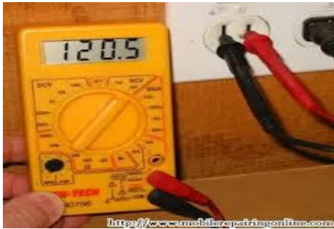
Fig. 4.12: Measurements of AC Voltage
