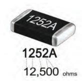
Fig. 1.16: Surface mount resistor
