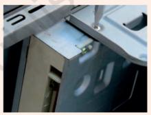
Fig. 2: Tighten screws of optical drive
