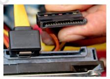
Fig. 12.40: Unplug 15-pin connector from HDD
