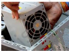
Fig. 12.50: Unscrew the SMPS and remove it from cabinet
