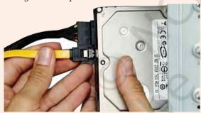
Fig. 5: Connecting SATA-data cable
