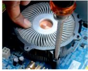
Fig. 12.7: Screw the heat sink
