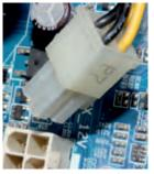
Fig. 12.46: Unplug 4-pin AUX power connector from power connector from motherboard
