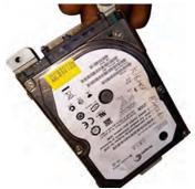
Fig. 12.63: Remove hard drive assembly
