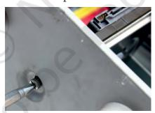
Fig. 12.51: Unscrewing of HDD
