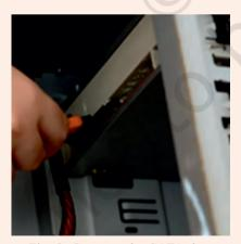
Fig. 3: Connect the SATA data cable
