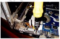
Fig. 12.71: DC power jack mounted under display hinge
