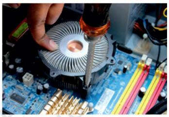
Fig. 12.44: Unscrew heat sink
