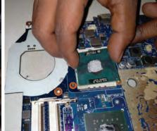
Fig. 12.57: Unscrew the socket
