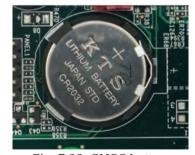
Fig. 7.23: CMOS battery
