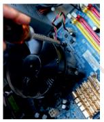
Fig. 12.8: Screw the heat sink fan assembly
