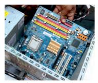
Fig. 12.10: Lay the motherboard over the standoffs
