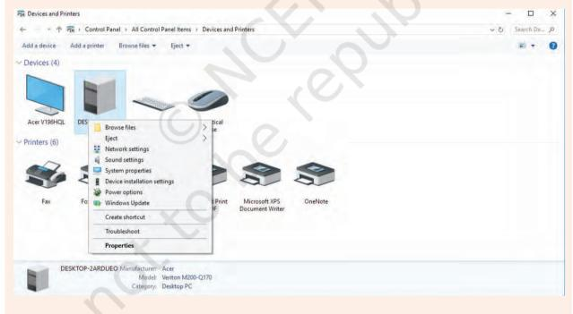
Fig. 1: Disabling the automatic device driver software installation
