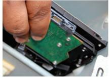
Fig. 12.52: Remove HDD
