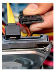
Fig. 12.20: Plug-in 15-pin connector to HDD
