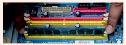
Fig. 1: Press down the memory in slot
