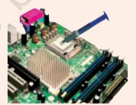
Fig. 2: Applying thermal compound on CPU
