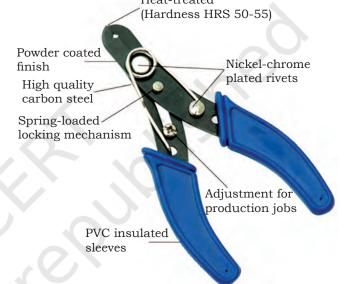
Fig.11.7: Wire stripper and its different parts
