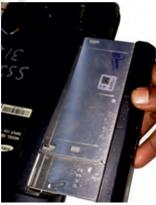
Fig. 12.67: Remove optical CD DVD drive connector board
