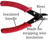
Fig. 11.2: Parts of electronic cutter
