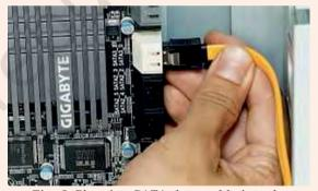
Fig. 6: Plugging SATA data cable into the motherboard
