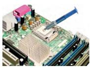
Fig. 12.6: Applying thermal compound on CPU
