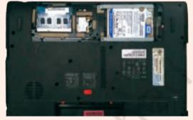
Fig. 1: Remove battery and optical drive
