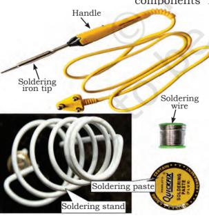
Fig. 1.32: Soldering kit
