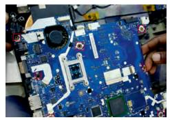
Fig. 12.73: Disconnect cables from motherboard and remove screws
