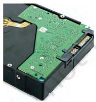
Fig. 10.15: Back of SATA HDD
