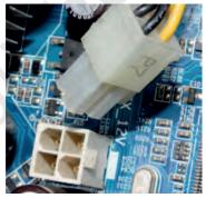
Fig. 12.19: Plug-in 4-pin AUX power connector to motherboard
