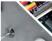
Fig. 12.13: Tighten screws of HDD
