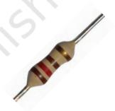
Fig. 1.17: (a) Fixed resistor
