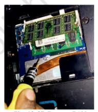
Fig. 12.65: Remove RAM memory modules
