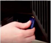
Fig. 12.22: Connecting VGA or monitor cable to the port on back panel of computer
