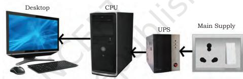
Fig. 12.29: Power connection (CPU through UPS)
