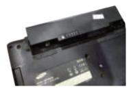
Fig. 12.59: Remove battery and optical drive
