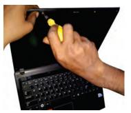
Fig. 12.77: Remove the four screws securing LCD screen
