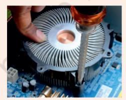
Fig. 1: Screwing the heat sink
