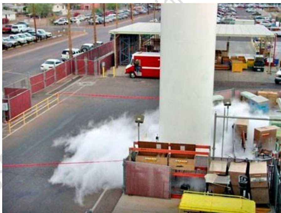
Fig. 4.6: An LH 2 leak will still make a visible cloud
