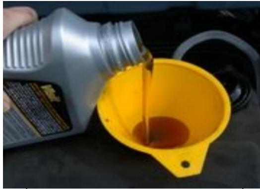
Fig. 3.6: Fill up oil with funnel
