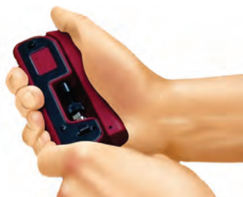
Fig. 9.16 Crimp the connector using a cable crimper
