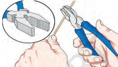
Fig. 9.30 Use a pair of pliers for bending the wire
