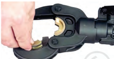
Fig. 9.69 Fixing the dies in crimper
