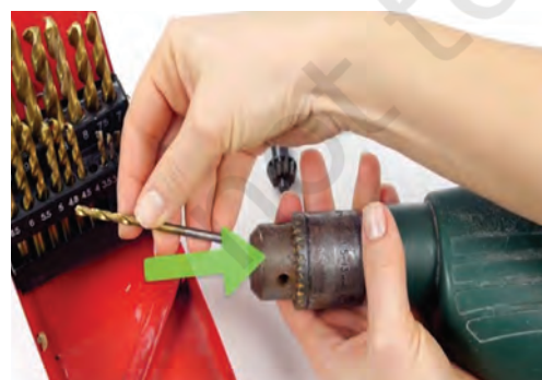
Fig. 7.23 Insert new drill bit
