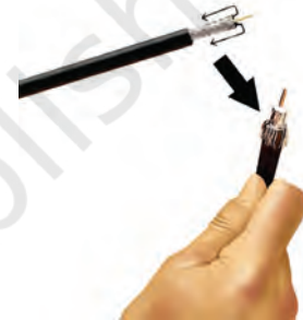
Fig. 9.13 Fold the ground wire of the cable
