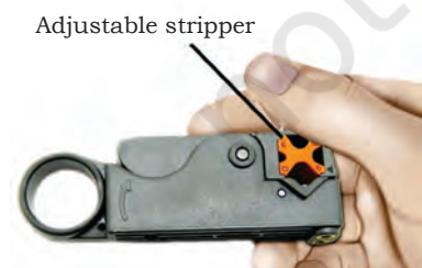
Fig. 9.9 Adjustable knob for stripper
