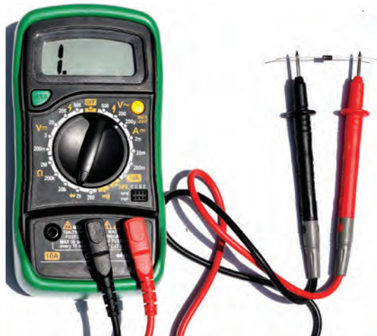
Fig. 2.32 Diode in reverse bias condition
