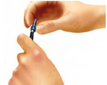
Fig. 9.15 Insert a connector in the cable conductor
