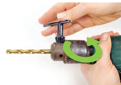
Fig. 7.21 Turn the chuck key counter clockwise
