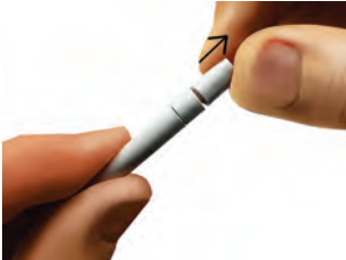
Fig. 9.11 Pull the outer shield of the cable
