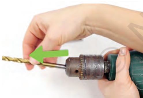
Fig. 7.22 Slide the drill bit out
