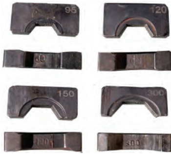
Fig. 9.59 Different size of dies used in hydraulic crimping tool (diameter of 95–300mm)
