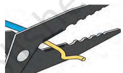
Fig. 9.25 Cut the damaged part of the wire
