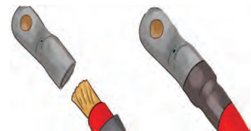
Fig. 9.66 Lugs connecting to the wire
