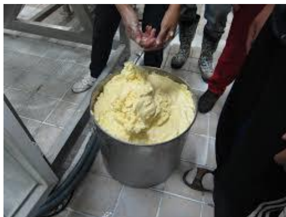
Fig. 3.3: Butter Formation During Cream Churning Process
