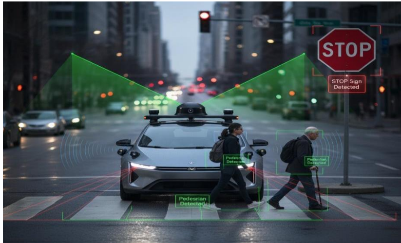
Fig. 2.11: Car detecting road signals and pedestrians using sensors
